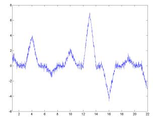
In this case, the wavelet coefficients should remove a first-order polynomial. If the signal value at an odd index, x(2n+1), is well approximated by a first-order polynomial fitted to the surrounding sample values, then 1/2(x(2n)+x(2n+2)) should provide a good fit for x(2n+1). In other words, x(2n+1) should be the midpoint between x(2n) and x(2n+2).
