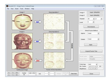
The synthesized image and its decomposition (which is equal to the fusion of the two decompositions) appear. The new image produced by fusion clearly exhibits features from the two original ones.
