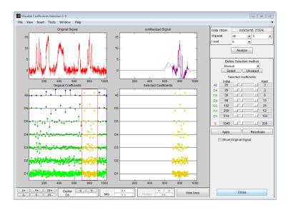
This illustrates that wavelet analysis is a local analysis since the signal is perfectly reconstructed around the position 800. Check the **Show Original Signal** to magnify it.
