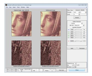
The tool displays its wavelet decomposition below the original image (on the left). The selected coefficients are displayed in the middle of the window, below the synthesized image (which, at this step, is the same since all the wavelet coefficients are kept). There are 11874 coefficients, a little bit more than the original image number of pixels, which is 96x96 = 9216.
