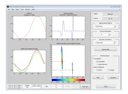
The running signal is the superimposition of two dilated and translated versions of the pattern F, namely F((t-20)/8) and F((t-40)/4). The two pairs (position, scale) to be detected are given by (20,8) and (40,4) and are materialized by dashed lines in the lower right graph of the contour plot of the CWT. The detection is perfect because the two local maxima of the absolute values of the continuous wavelet coefficients fit perfectly.
